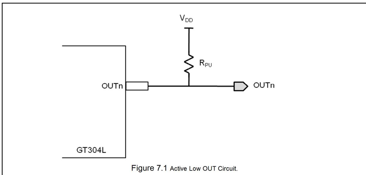
Figure 7.1 Active Low OUT Circuit.
