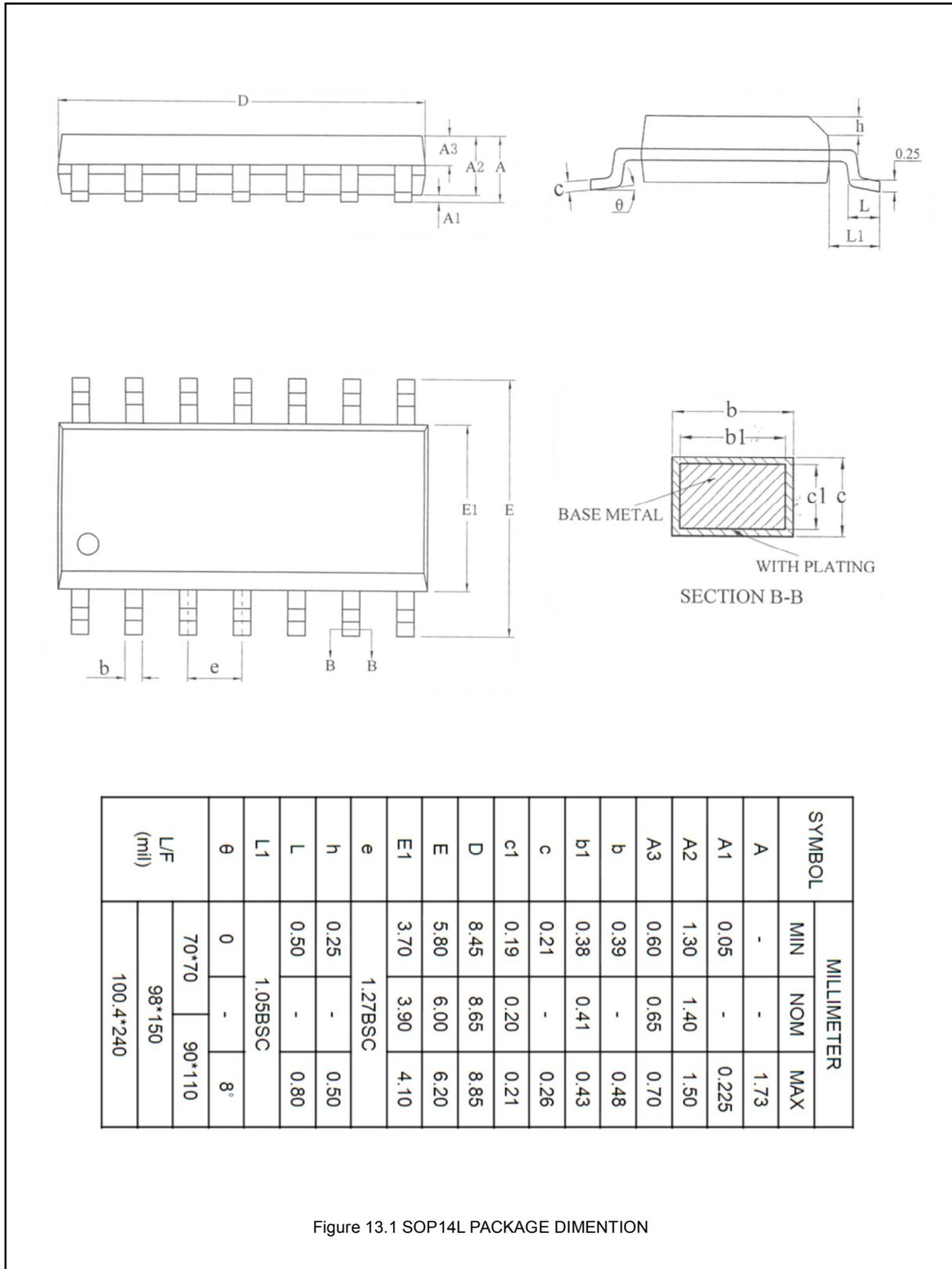
Figure 13.1 SOP14L PACKAGE DIMENTION
