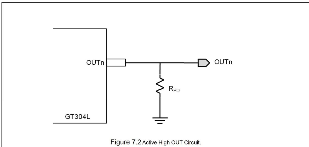
Figure 7.2 Active High OUT Circuit.
