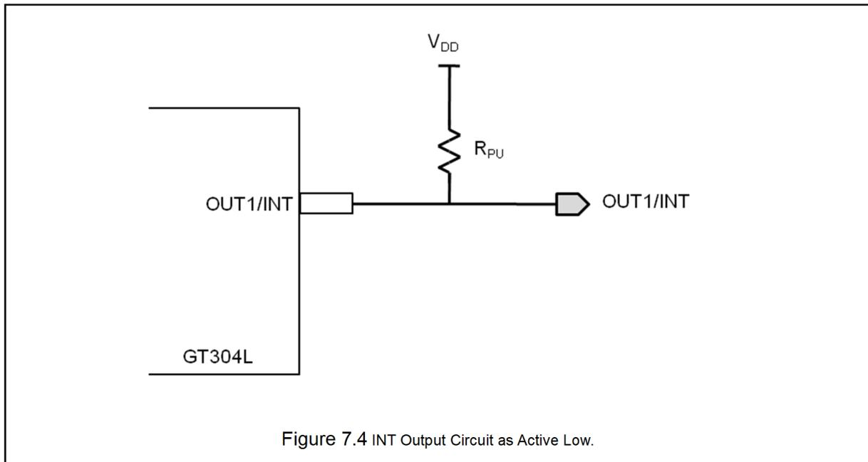
Figure 7.4 INT Output Circuit as Active Low.
