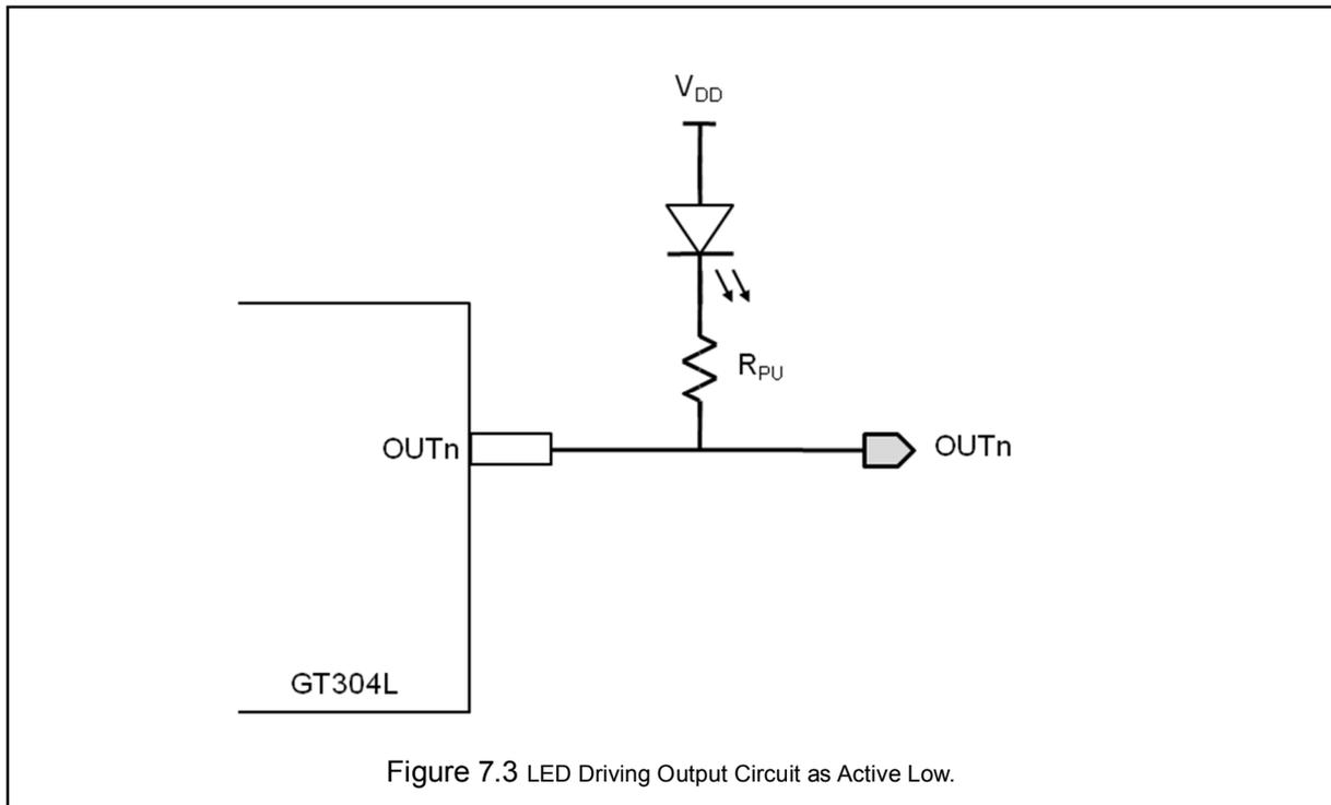
Figure 7.3 LED Driving Output Circuit as Active Low.
