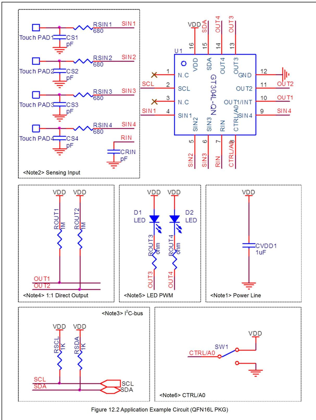
Figure 12.2 Application Example Circuit (QFN16L PKG)
