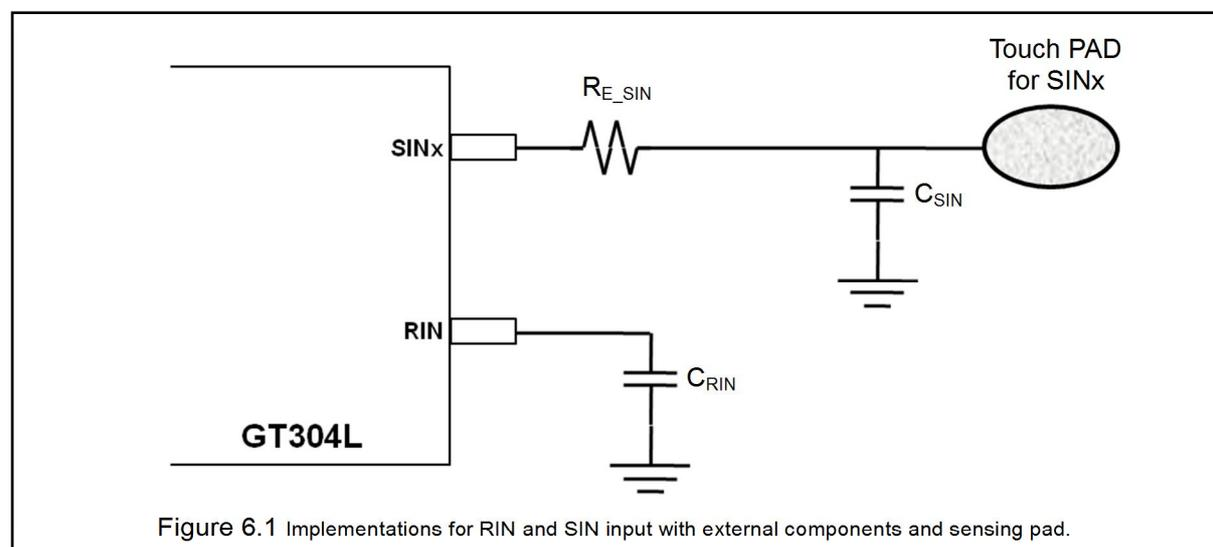
Figure 6.1 Implementations for RIN and SIN input with external components and sensing pad.
