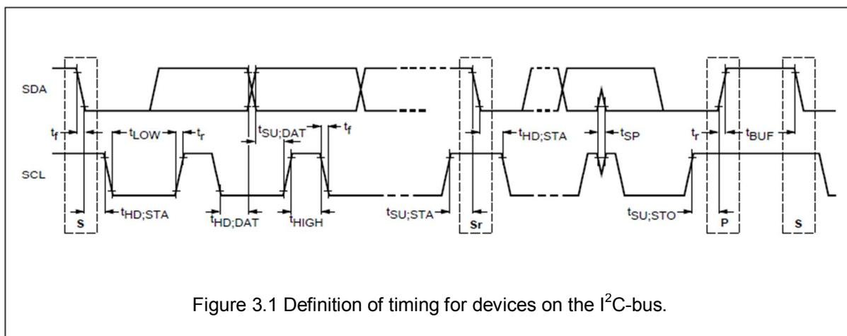
Figure 3.1 Definition of timing for devices on the I<sup>2</sup>C-bus.
