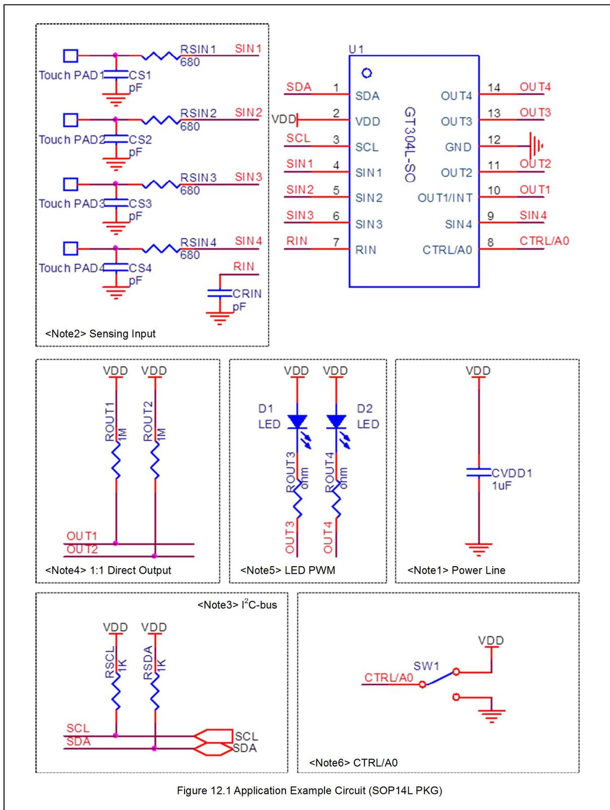
Figure 12.1 Application Example Circuit (SOP14L PKG)
