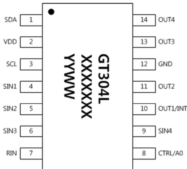
Figure 4.1 SOP14L Pinout Diagram (Top View)
