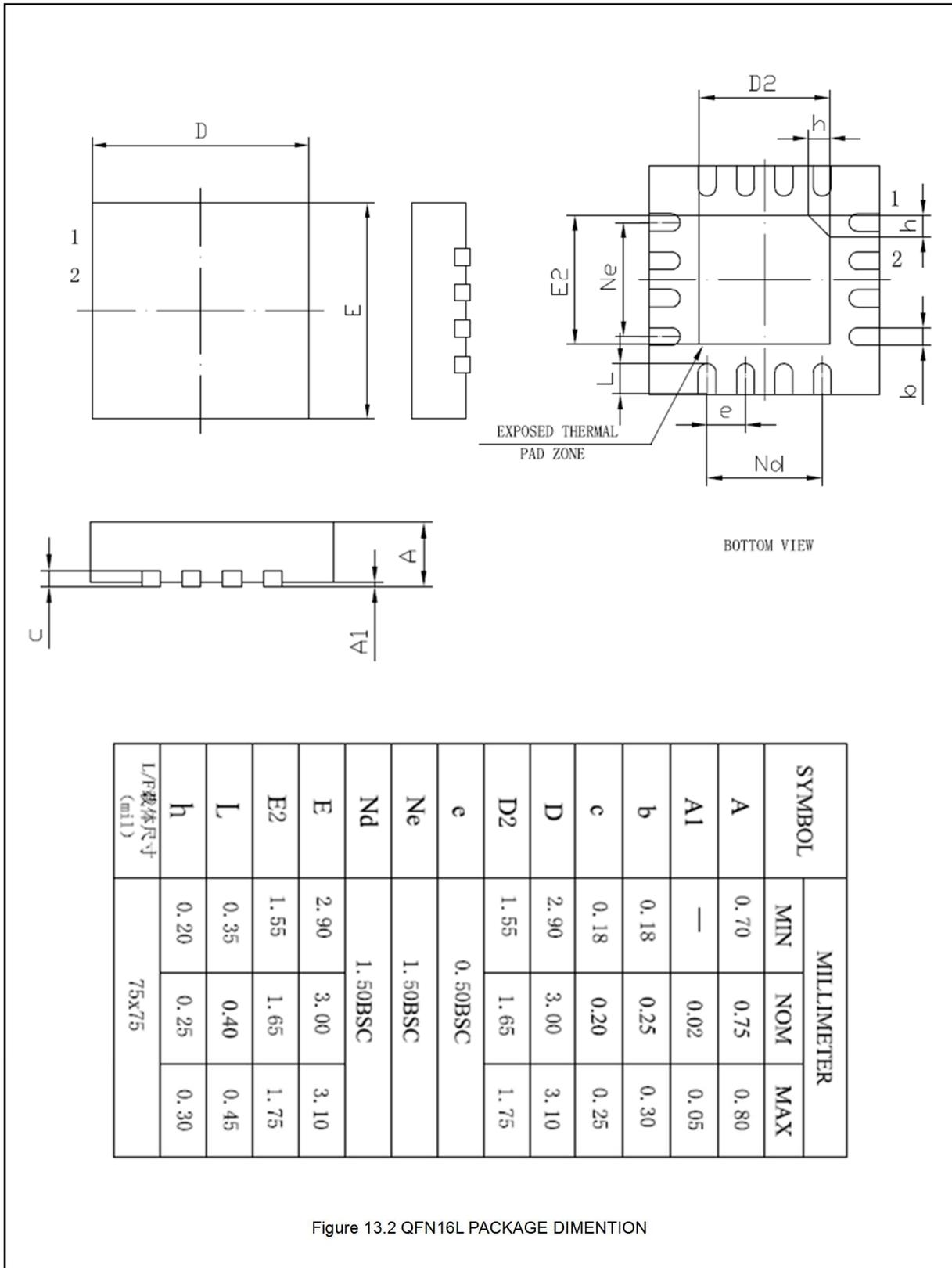
Figure 13.2 QFN16L PACKAGE DIMENTION
