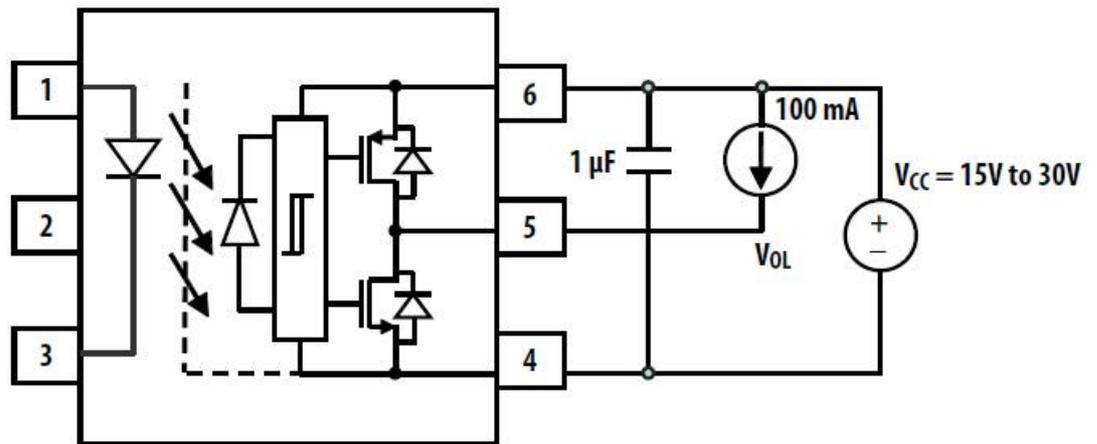
**Fig.18 IFLH Test Circuit**
