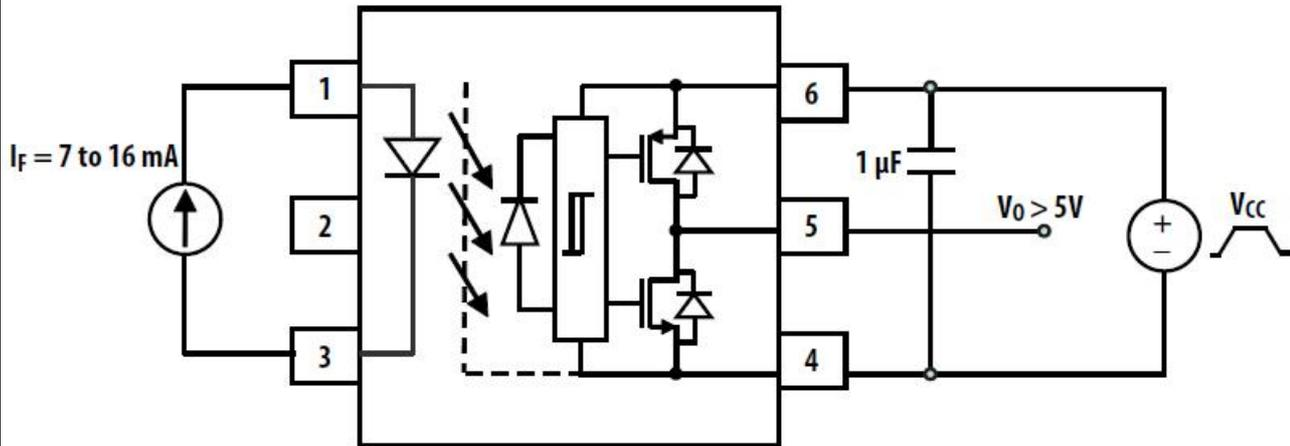
**Fig.20 t<sub>PHL</sub>, t<sub>PLH</sub>, t<sub>r</sub> and t<sub>f</sub> Test Circuit and Waveforms**
