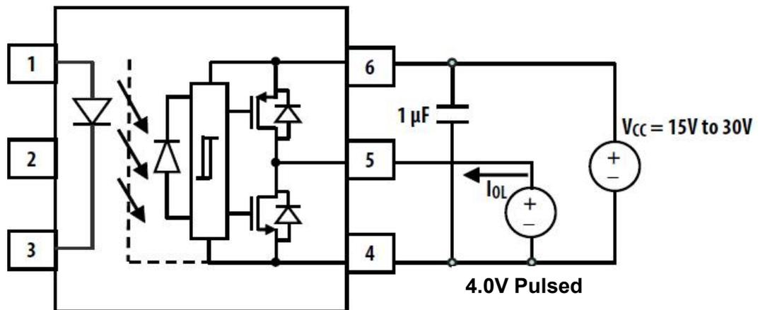
**Fig.16 VOH Test Circuit**
