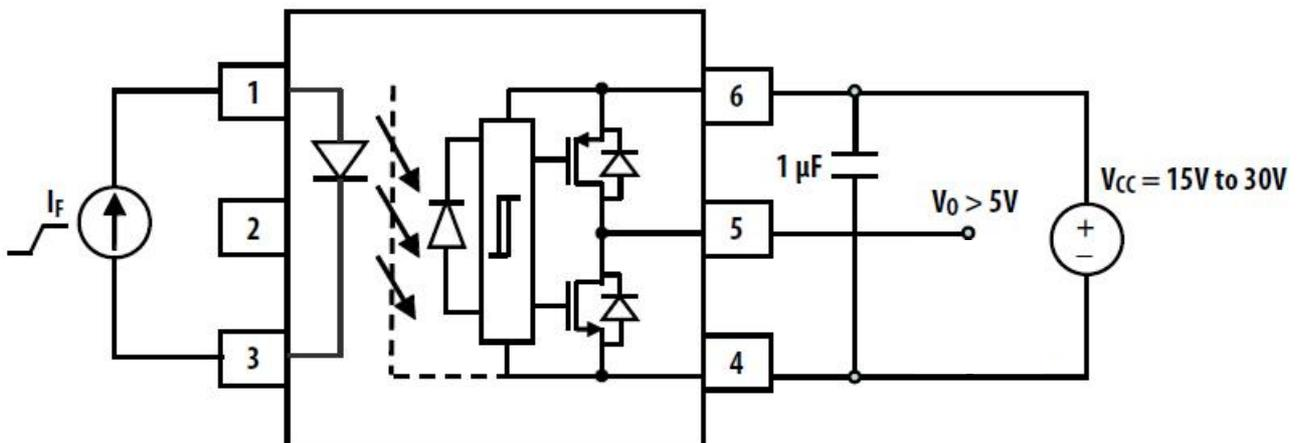
**Fig.19 UVLO Test Circuit**
